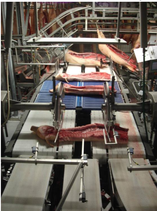
Fig. 1. An automated cutting line. The half carcass is cut into three primals: Ham, Middle and Shoulder.
