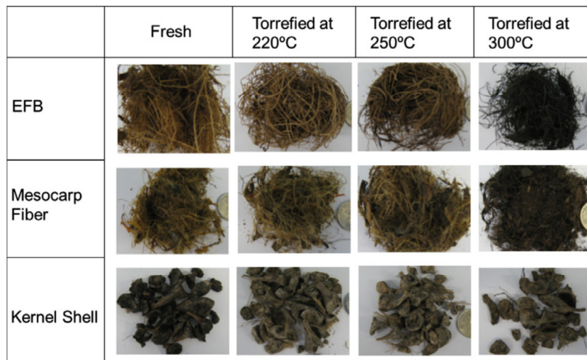
Figure 2. Images of Empty fruit bunches, mesocarp fiber and kernel shell after torrefaction at 220, 250 and 300 °C (Uemura et al, 2011).
