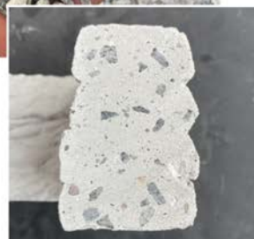
Concrete ( \varnothing_{\max} = 8\text{mm} )
