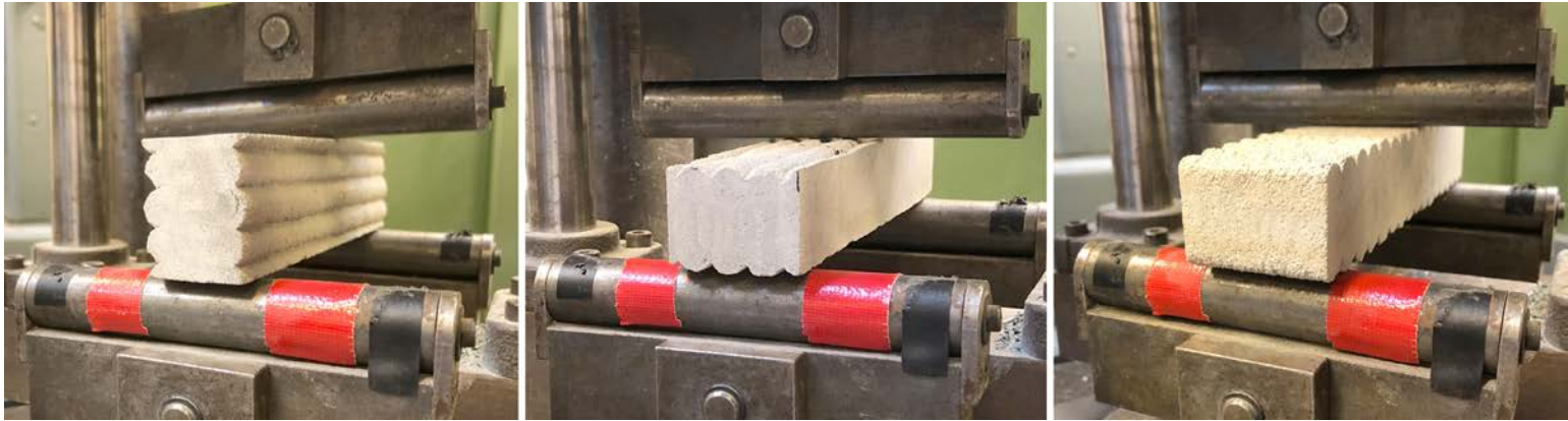
Mechanical flexural tensile testing of 3D printed concrete specimens. This type of test is typically performed in 3 different directions to quantify the influence of the layered structure and printing direction. The specimen is subjected to three-point bending and the ultimate load is recorded and converted into a tensile strength.
