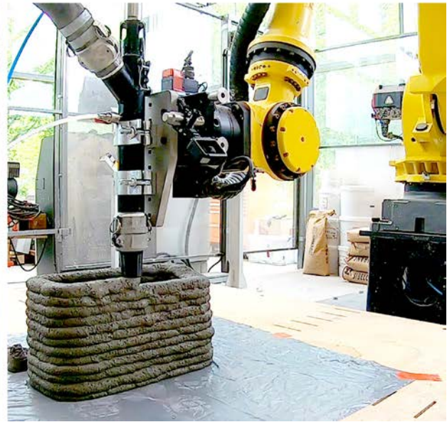
Left: Print with mortar (max. particle size 1mm. Right: Concrete print (max. particle size 8 mm.
