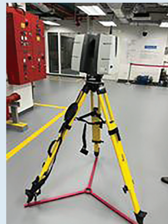
FIGURE 12. 3D LASER SCANNER AT THE IBEC ENABLING 3D SCANNING OF BUILDINGS
